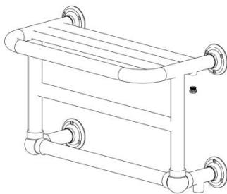
2. Measure the distance between all the location holes and mark these on the wall in the required location, use a spirit level to ensure these are horizontally and vertically aligned.
