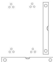
3. Position the towel rail and screw into place using the screws provided.
