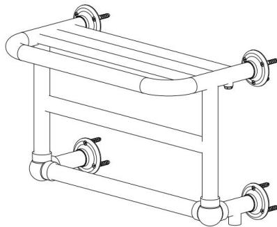
5. Finally, fit the radiator valves to the pipework and connect to the radiator valve tail and tighten all connections.
